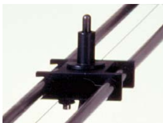
Vertical probe holder for mounting the ion chamber towards the beam source.
