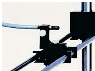
Indexed probe holder for mounting the ion chamber perpendicular to the beam. The ion chamber may be fixed in any scan direction including at 45 degrees diagonal to the scanning mechanism.
